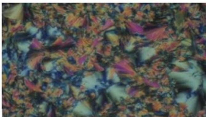
Figure 1. POM micrograph of the salt with n = 8 shows the smectic LC phase taken at 150 °C (magnification 400x).
